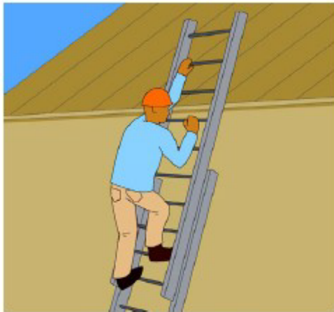
Figure 2: Ladder extending three feet above the landing area.
